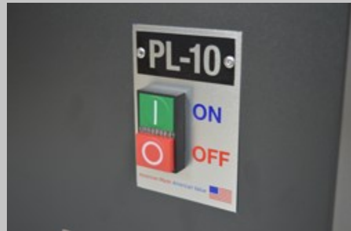
Built-In Motor Starter with Start / Stop Switch
